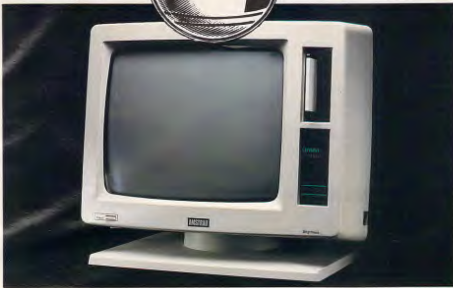
The disk drives: a 720k disk drive is available as an optional extra
